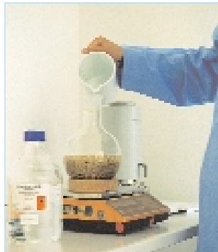
Distilling chamomile flowers to extract the essential oil: respective filled weights of chamomile flowers and water (left), and assembling the distillation equipment in the laboratory
